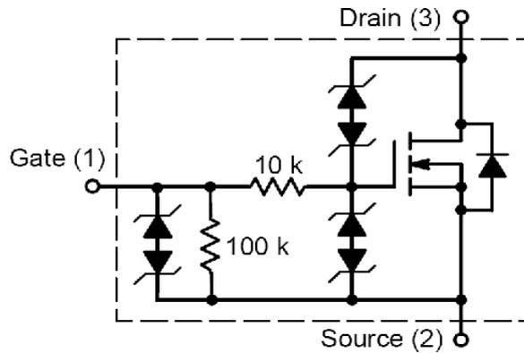
Figure 10. Digital Output Internal Drive Circuit
