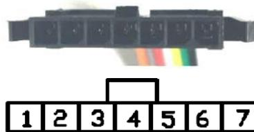
Figure 4. 7-pin Connector of the IQL 4G
