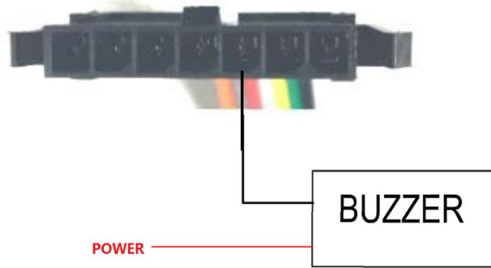
Figure 11. Typical Connection with a Buzzer as Digital Output
