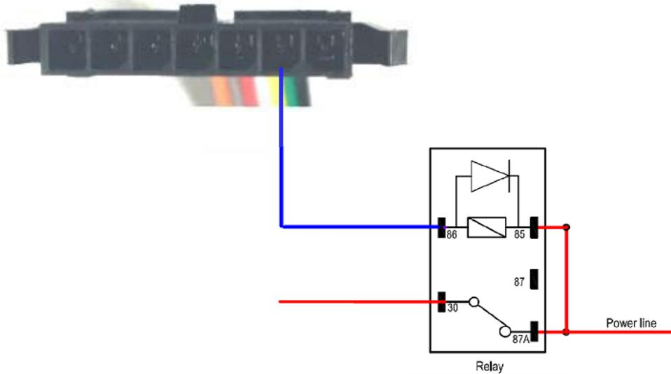
Figure 14. Typical Connection with a Relay
