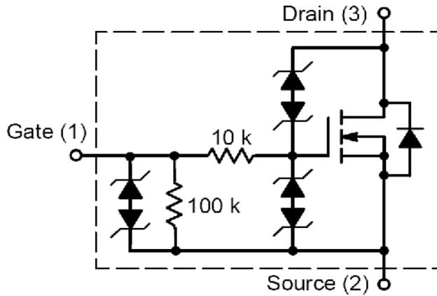
Figure 13. Digital Output Internal Drive Circuit
