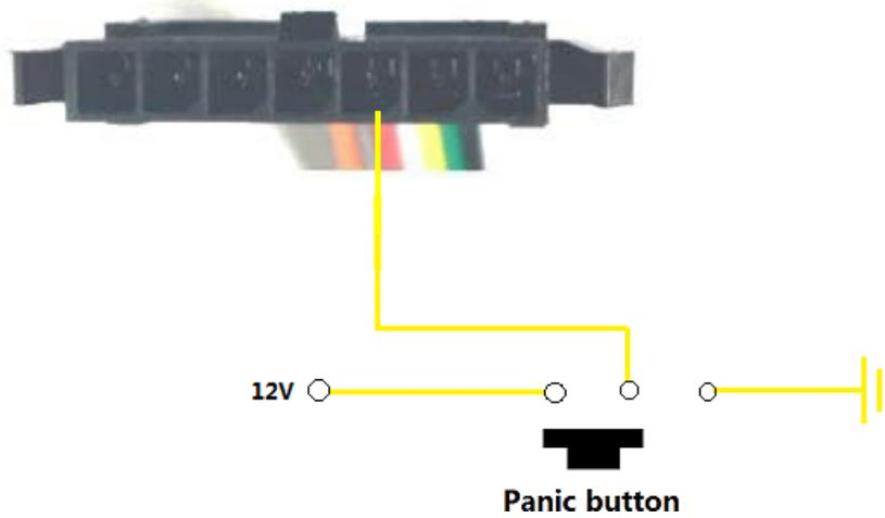
Figure 12. Typical Digital Input Connection
