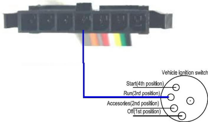
Figure 9. Typical Ignition Detection
